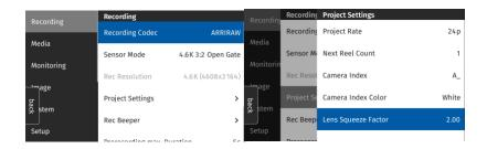
Since we are using a 2.0x anamorphic lens, we set the lens squeeze factor to 2.00. We decided to use a 5% safe area for stabilization and reposition, therefore we must generate a custom 2.39:1 frame line with 95% scaling (100% - 5% = 95%) for a lens squeeze of 2.0x. This can easily be achieved by using the <u>Frame Line</u> & Lens Illumination Tool on our website.
