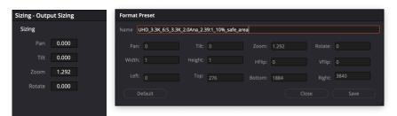
Since our target aspect ratio is 2.39:1 this will result in an active image of 2.39:1 with letterbox inside the UHD container, which is 1.78:1. In this case we don't have to add an additional crop, since the image is already
