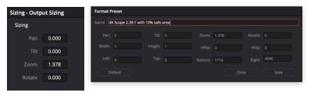
This will result in correctly framed image inside our target resolution and aspect ratio, which is 4K scope with 4096x1716 pixels. Since there is a 10% safe zone it is still possible to slightly adjust the image with a pan, tilt or zoom.
