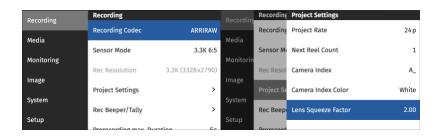
Since we are using a 2.0x anamorphic lens, we set the lens squeeze factor to 2.00. We decided to use a 10% safe area for stabilization and reposition, therefore we must generate a custom 2.39:1 frame line with 90% scaling (100% - 10% = 90%) for a lens squeeze of 2.0x. This can easily be achieved by using the Frame Line & Lens Illumination Tool on our website.
