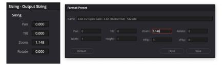
This will result in correctly framed image inside our target resolution and aspect ratio, which is 4K scope with 4096x1716 pixels. Since there is a 5% safe zone it is still possible to slightly adjust the image with a pan, tilt or zoom.
