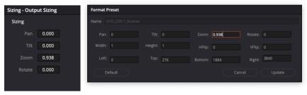
Since our target aspect ratio is 2.39:1 this will result in an active image of 2.39:1 with letterbox inside the UHD container, which is 1.78:1. For a correct 2.39:1 letterbox we must set a crop for 2.39:1 here, which results in Top = 276 and Bottom = 1884 pixels/lines.
