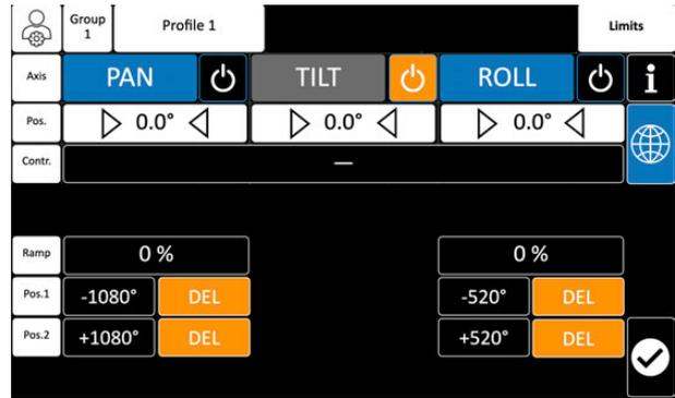
Or tap a position value in the first and second line, which will highlight the field in green, and then utilize one of the jog wheels to move until the desired position value is established.
