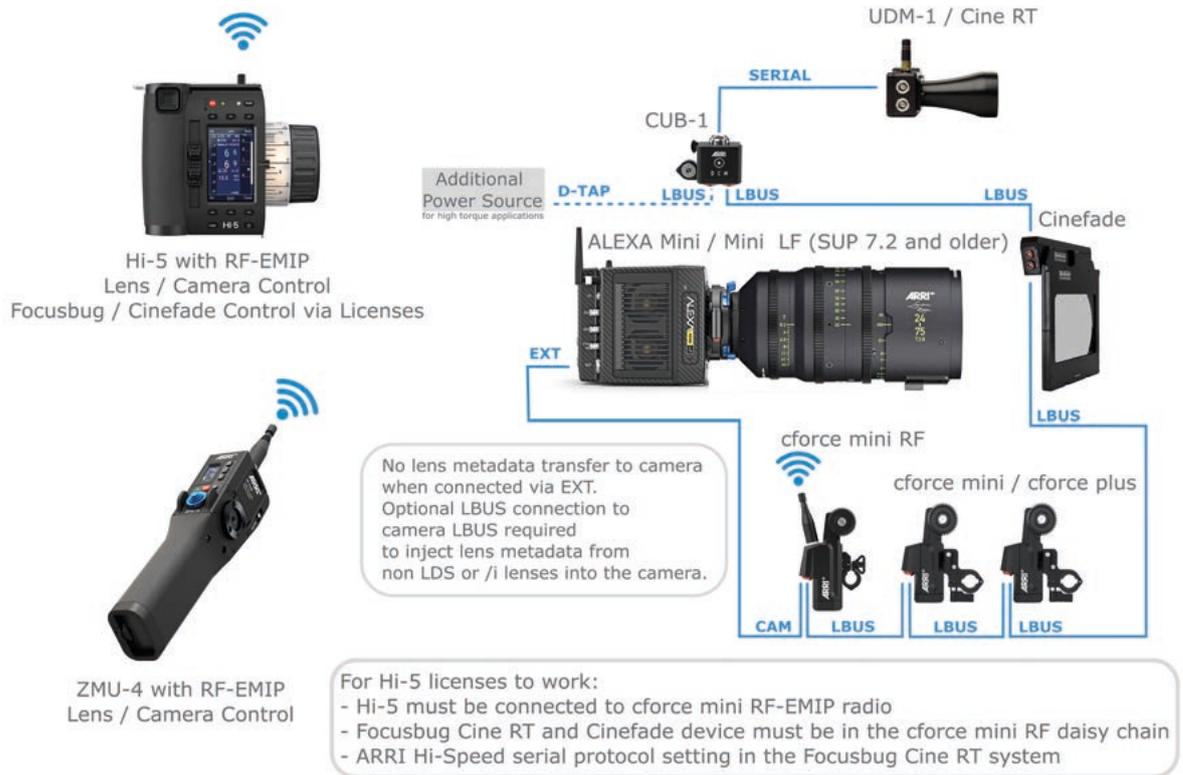
6) Focusbug and Cinefade with a cforce mini RF as a radio host on an ALEXA Mini or ALEXA Mini LF (SUP 7.2 or older)
