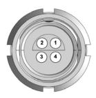
Pin 1 NC Pin 2 Ground Pin 3 NC Pin 4 Trigger
