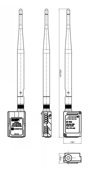
Weight of the RF-900 Radio Module: 55g/1,94oz (including antenna)
