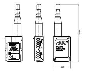
Weight of the RF-2400 Radio Module: 52g/1,83oz (including antenna)
